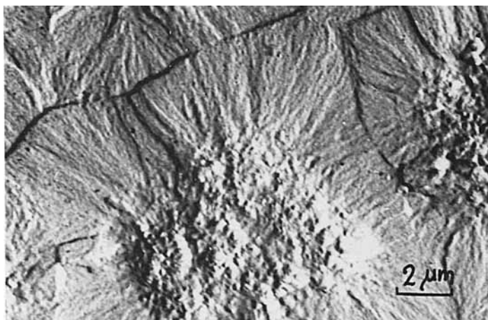
Fig. 2. Granular aggregates of type II in sample PU 2 (replica of fracture surface).
