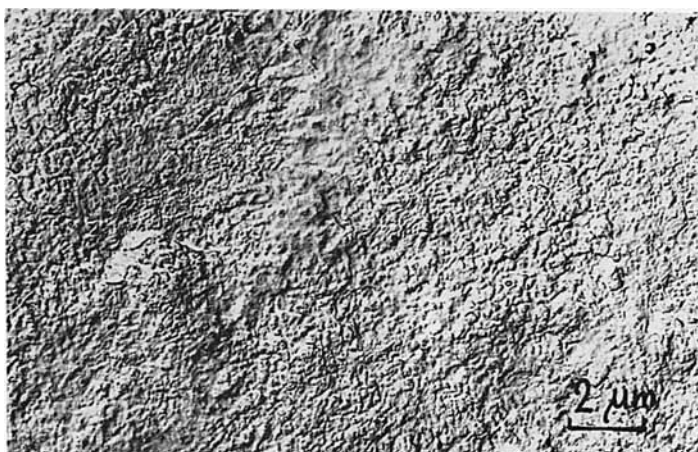
Fig. 5. Larger number of granular elements in sample PU 5 (replica of fracture surface).
