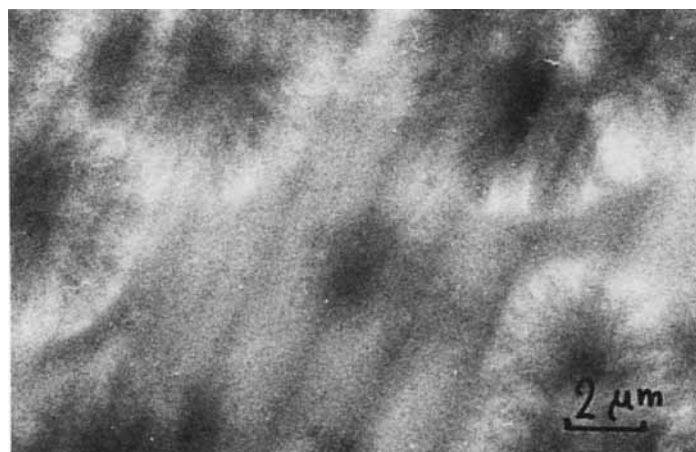
Fig. 8. Structural elements in a thin section, cutting temperature 150 K.
