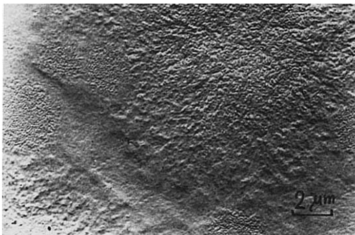
Fig. 4. Different structure of the continuous phase in sample PU 4 (sample PU 3 after annealing at 425 K for 5 h) (replica of fracture surface).
